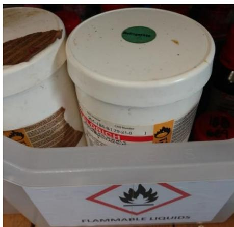
The photograph shows some peroxyacetic acid (an oxidising agent) which had been incorrectly placed in a flammables store. Getting this wrong, as happened here, is an easy way to cause fires. Please make sure you know the difference between the flammable and oxidising hazard labels. Flammables have a flame whilst oxidising agents have a flame above an O.
